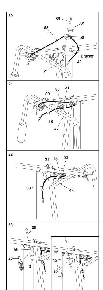
24. See the inset drawing. Attach a 3 1/2" Pulley (15) and a Cable Trap (66) to the upper hole in a Long "U"-Bracket (57) with a 3/8" x 2" Bolt (12) and a 3/8" Nylon Locknut (21). Be sure that the Cable Trap is inside the Long "U"-Bracket. Note: This may come pre-assembled.
